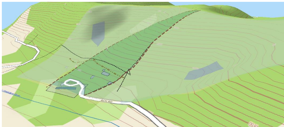
figure 2. 3-D view of site and hillside above from south. (blue arrows indicate potential drain paths during intense rain)
